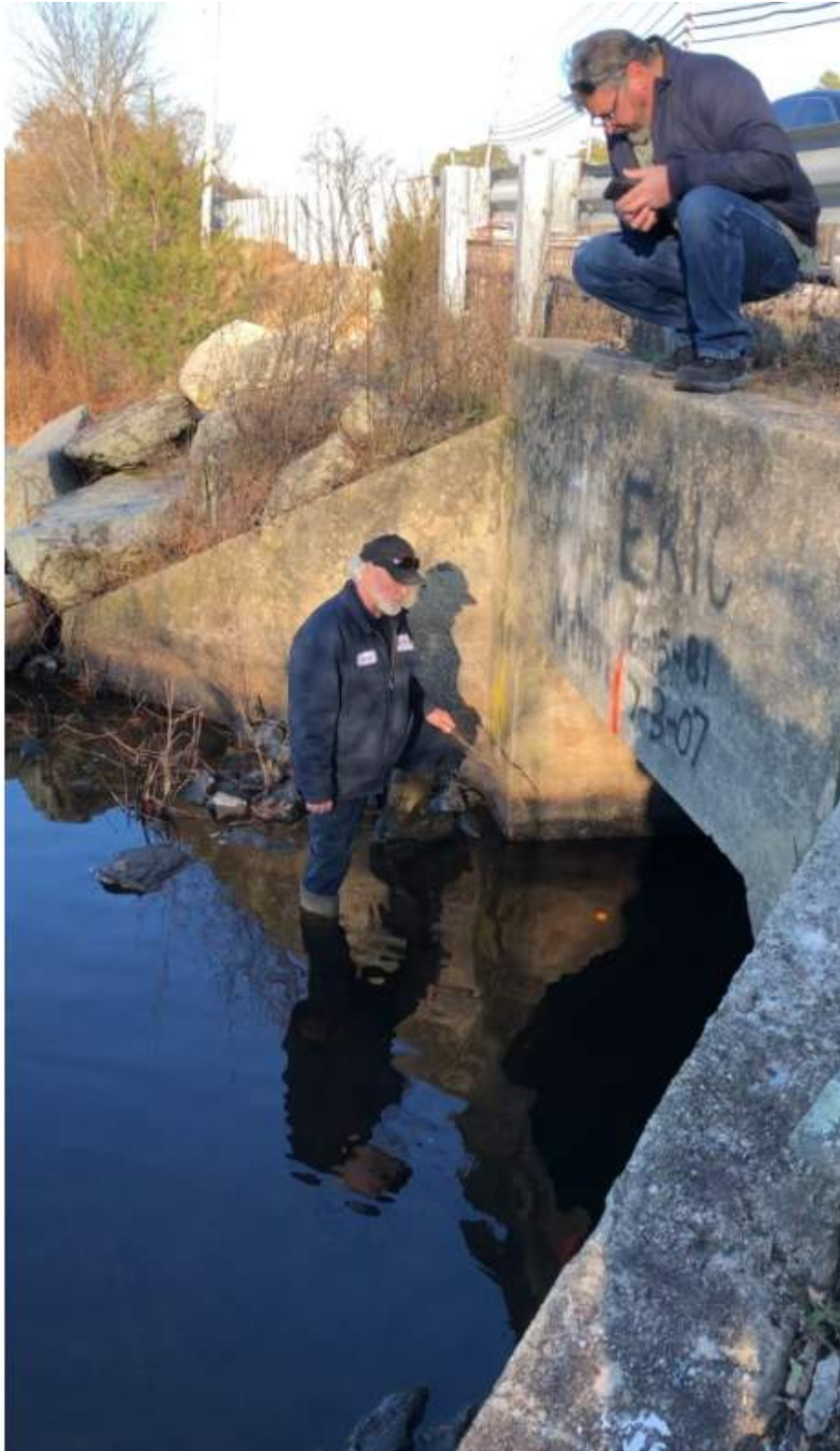
Figure 4-3. Estimating Surface Velocity Using an Orange
